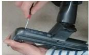
(5) Disassemble the side decor as shown in the photograph.
