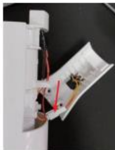
(2) Disassemble the parts and disconnect the marked connectors.
