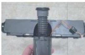
(14) Disassemble the hose as shown in the photograph.
