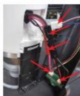
(3) Disconnect the 5 marked connectors out of the five connected harnesses.
