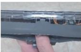
(13) When disassembling the cover and wire, you will find they are sturdily fastened with hooks.
