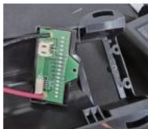
(4) Disassemble one screw (M2.6*8) located at the bottom of the Pin PCB.
