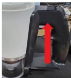
(2) Disassemble by pulling the handle in the direction indicated.
