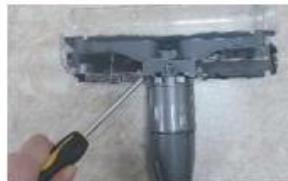
(12) Disassemble the cover and wire as shown in the photograph.
