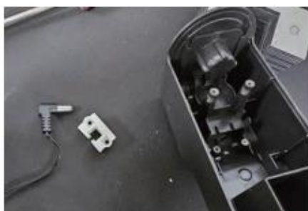
(5) Separate the adapter and adapter fixing parts.
