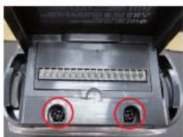
(1) After disassembling the battery, disassemble the two screws (M3*8) on the handle side.
