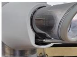
(4) Disassemble the cover pipe using a tool such as a flat-blade screwdriver.
