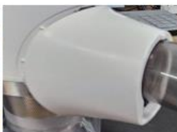
(4) Disassemble the cover pipe using a tool such as a flat-blade screwdriver.
