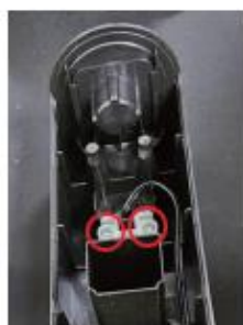
(4) Disassemble the 2 marked screws.
