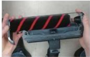
(1) Disassemble the nozzle roller. (For a detailed disassembly method, refer to How to Disassemble the Nozzle Roller.)
