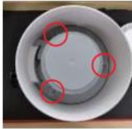
(5) Disassemble the three screws (M3*10)
