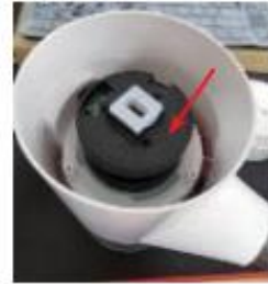
(6) Separate the motor from the main body.
