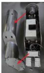
(2) Separate the 2 marked parts from the charging Station.
