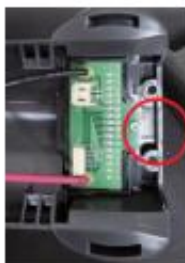
(4) Disassemble one screw (M2.6*8) located at the bottom of the Pin PCB.
