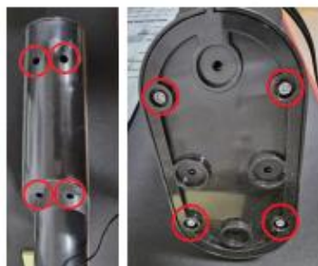
(1) Disassemble the 8 marked screws.
