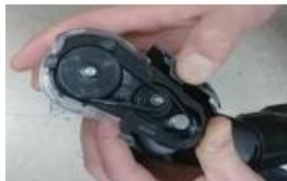
(10) Lift the cover decor and disassemble the motor assembly.
