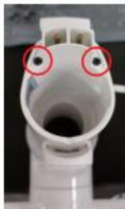
(1) Disassemble the 4 marked screws.
