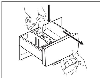
2. Remove the top part of the additive compartment to aid cleaning and flush it out under running warm water, to remove any traces of accumulated detergent.
