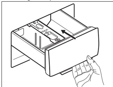
Make sure that the detergent divider is inserted properly and does not cause a blockage when you close the drawer.
