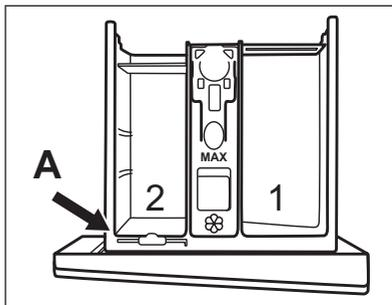
2. **To use also liquid detergent/additive or bleach:** Remove detergent divider from the position **A** and insert it in position **B**.
