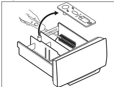
3. Make sure that all detergent residue is removed from the upper and lower part of the recess. Use a small brush to clean the recess.
