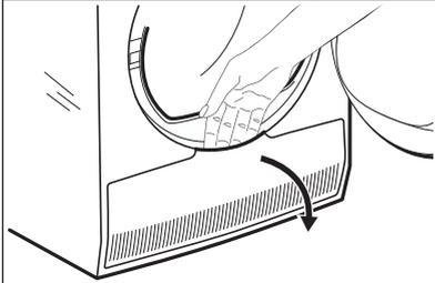
3. Turn the levers to unlock the condenser lid.
