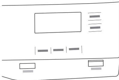
To activate or deactivate an option touch the relevant button or a two button combination. Corresponding symbol on the display or the led above the button lights up.
