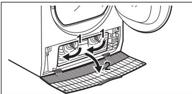
4. If necessary, remove the fluff from the condenser and its compartment. You can use a vacuum cleaner with a brush attachment.
