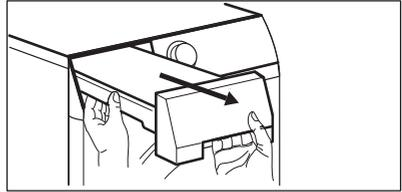
2. Pull the plastic connection out and drain the water into a basin or equivalent receptacle.
