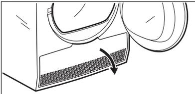
3. Turn the levers to unlock the condenser lid and lower the condenser lid. .
