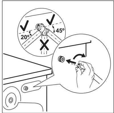
2. Position it toward left or right depending on the position of the tap. Make sure that the inlet hose is not in vertical position.
