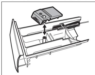
3. Flush the detergent drawer out under running warm water to remove any traces of accumulated detergent. After cleaning, replace the top part in its position.
