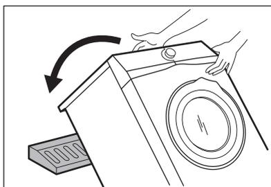
7. Remove the protection from the bottom.
