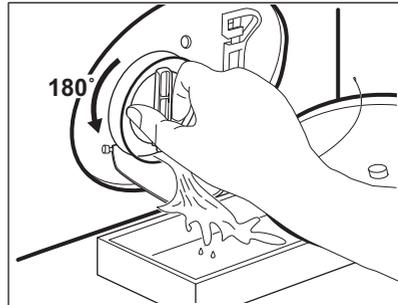
5. When the bowl is full of water, turn the filter back and empty the container.
