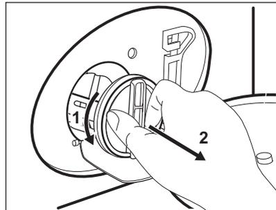
8. If it is necessary, remove fluff and objects from the filter recess.
