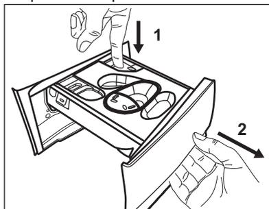
2. Remove the container for liquid detergent, if inserted.
