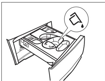
c) Put the **tablets** in the compartment
