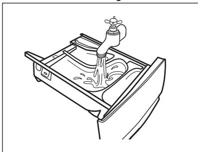
5. Make sure that all detergent residue is removed from the upper and lower part of the recess. Use a small brush to clean the recess.
