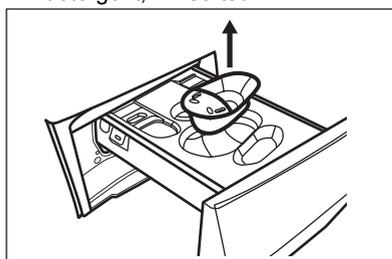
3. Lift up the top cover of the compartments to remove it.
