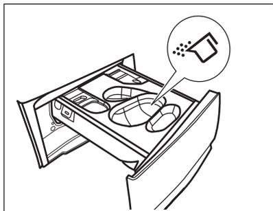
b) Pour the **liquid detergent** in the same compartment after inserting the relevant container
