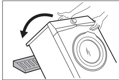
7. Remove the protection from the bottom.
