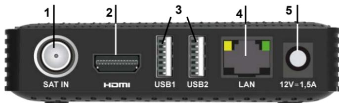
1. **SAT IN:** for connecting the satellite antenna (dish).
