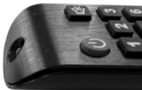
On the TV remote control, press and hold the button to be set (e.g. **VOL+**) until the red led remains steady. Press the **SET** button to save. Set one button at a time.
