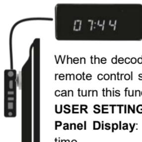
When the decoder is turned off (standby), the remote control sensor displays the time. You can turn this function off by entering the menu **USER SETTINGS > Standby Setting > Front Panel Display**: select *Off* to not display the time.
