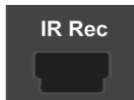
7. **IR:** for connecting the IR sensor of the remote control, to be placed on the front panel of the TV. The IR sensor has a standby time display that can be turned off.
