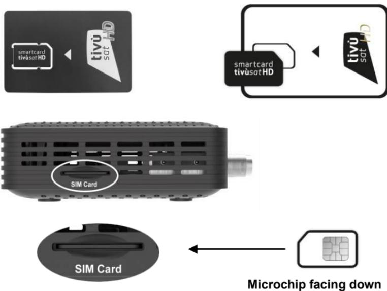
If you need to remove the SIM, push down to the click to unhook it and pull it out.
