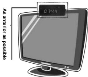
**Note:** The sensor is transparent and can receive the signal from multiple angles.
