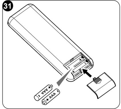
The remote control uses two dry alkaline 1.5V batteries (AAA.LR03) (fig. 31). When the batteries have been replaced, adjust the remote control clock.
