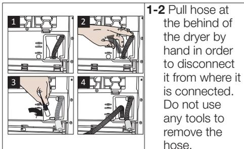
**1-2** Pull hose at the behind of the dryer by hand in order to disconnect it from where it is connected. Do not use any tools to remove the hose.
